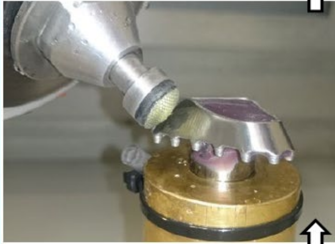
(b) Nickel bonded 40 \mu\text{m}
